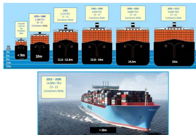
Figure 3. The level of sea depth affects the cargo volume of a cargo ship
